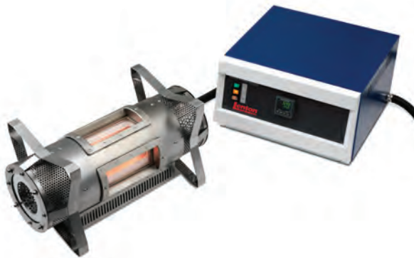
Vertical / horizontal tube furnace with 4 quartz viewing windows.
