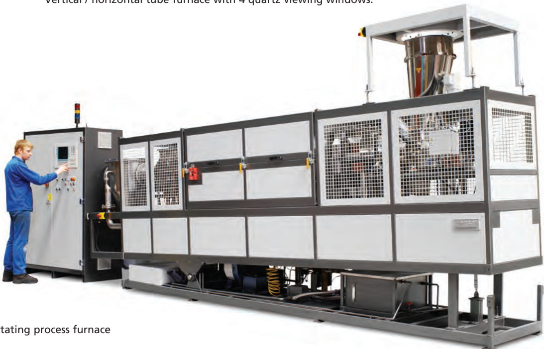
Vertical / horizontal tube furnace with 4 quartz viewing windows.
